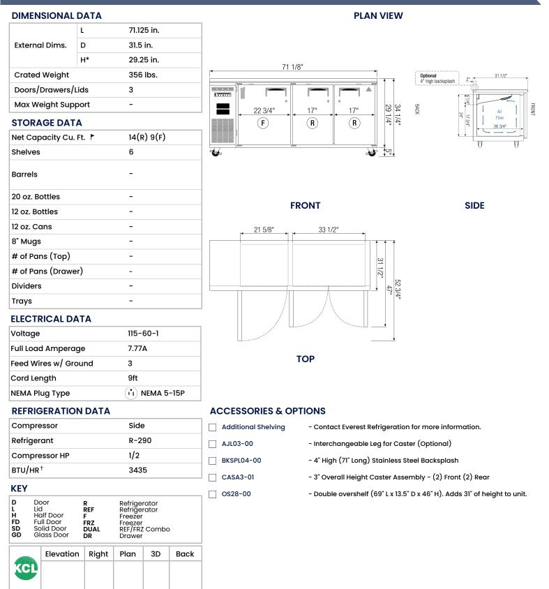
(†)Based on evaporating temperature of 23°F (~5°C) & condensing temperature of 131°F (55°C). ( ) Product capacity is calculated based on standard industry figures. (\*) Reference plan view for clarification on caster/unit height. If dimensions and capacity are critical, please contact Everest Refrigeration. Blizzard R290 replacement is at the sole discretion of Everest Refrigeration. Specifications subject to change without notice.
