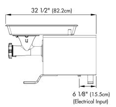
**Motor:** 1 hp grease packed gear motor provides compact, smooth, and quiet performance with an 8:1 reduction within the gear motor resulting in a 224RPM drive shaft output. Worm is coupled directly with the gear output shaft.
