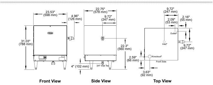
Outlet, Inlet, and Knockout are located on the bottom of unit.
