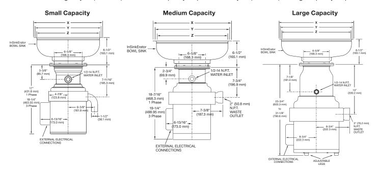
If mounting directly to a sink, use dimension chart below for adaptor height in place of InSinkErator bowl sink height. *IMPORTANT:* #5 adaptors only available on small and medium capacity disposers.
