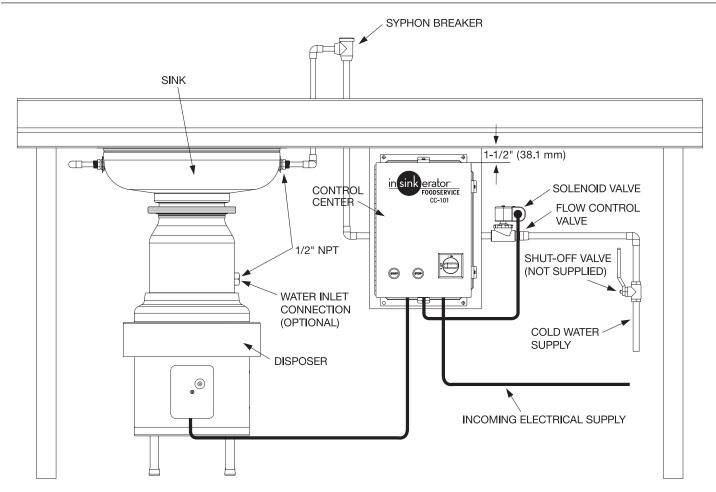
NOTE: The CC-101 control center should be mounted 1-1/2" (38.1 mm) back from the front surface of the table.
