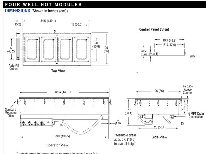
Controls must be mounted on operator (raceway) side for proper orientation with wells.
