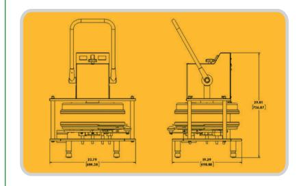
Electrical Data: 220v/50-60hz, 3200w, 1 Phase Temperature Range: 0 - 400° F (0 - 205° C) Construction: All Stainless Steel Shipping Weight: 225 lbs. (102.3 kgs)
