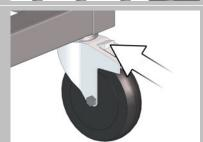
Release the transport trolley's parking brakes.
