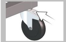
Release the transport trolley's parking brakes and move the trolley in front of the combi oven.
