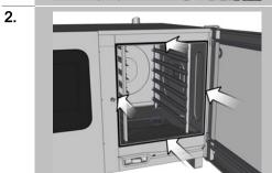
Once all four corners are in place, meticulously press the hygienic plug-in gasket into the rest of the guide.
