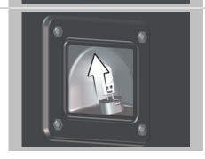
Reach into the reflector housing through the opening on the oven wall and pull out the halogen lamp upwards in a straight line.
