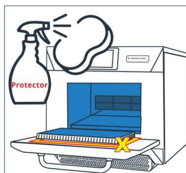
7. Apply oven protector (optional). Spray Merrychef Protector onto a sponge and spread lightly onto the sides of the inside of the oven, the back, the base, the roof and the oven door and heat oven afterwards.
