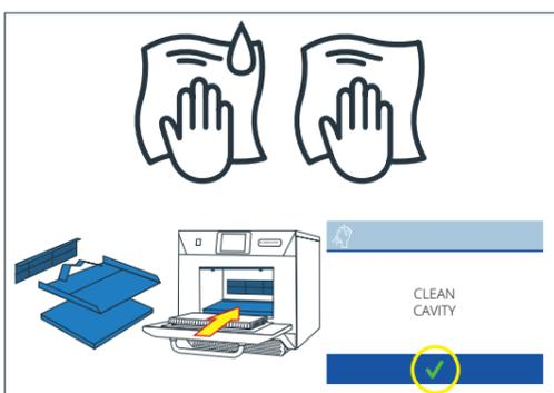
6. Remove the Merrychef cleaner with a clean wet cloth. The door seal can also be gently wiped if necessary to remove food debris.
