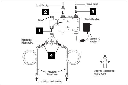
side of the hot water supply line to the hot side of the mixing valve and tighten properly and do the same for the cold supply line. Do not overtighten. Do not use thread sealant.
