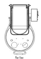
Line drawing is the SL300RB SL250RB SL300RB Α 52 7/8" (134.3cm) 52 7/8" (134.3cm) В **79 1/4"** (201cm) **79 1/4"** (201cm) C 58 3/8" (148.1cm 58 3/8" (148.1cm 89 7/8" (228.1cm) 89 7/8" (228.1cm) 76 1/2" (194cm) 76 1/2" (194cm)
