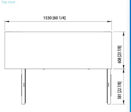
2 Doors Capacity 15.6 Cu.Ft. **Shelves** 4 Refrigerant R-290 **Temperature** 33°F ~ 39°F Range Easy Sliding Maintenance **Condensing Unit** 9.8 ft long (3m) flexible three Connection wire cord with modeled plug HP 3/8 Voltage 115V/60Hz **Amps** 3.5 **NEMA Config.** NEMA 5-15 Lighting Interior LED lighting
