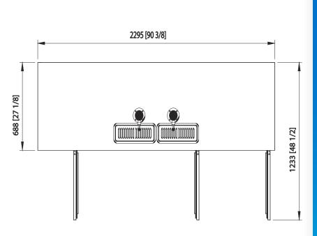
Barrels(1/2) Capacity 31.5 Cu.Ft. Doors 3 Refrigerant R-290 **Temperature** 33°F ~ 39°F Range Easy Sliding Maintenance **Condensing Unit** 9.8 ft long (3m) flexible three Connection wire cord with modeled plug HP 3/8 Voltage 115V/60Hz **Amps** 3.8 **NEMA Config.** NEMA 5-15 Lighting Interior LED lighting
