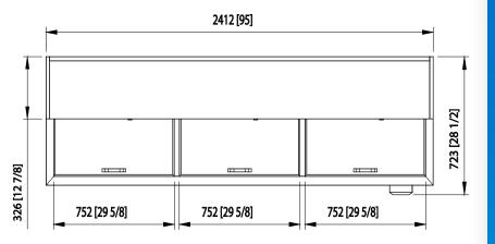
3 **Doors** Capacity 31.3 Cu.Ft. **Dividers** 5 Refrigerant R-290 **Temperature** 33°F ~ 39°F Range Easy Sliding Maintenance **Condensing Unit** 9.8 ft long (3m) flexible three Connection wire cord with modeled plug HP 3/8 Voltage 115V/60Hz **Amps** 3.5 **NEMA Config.** NEMA 5-15
