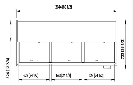
3 **Doors** Capacity 26 Cu.Ft. **Dividers** 4 Refrigerant R-290 **Temperature** 33°F ~ 39°F Range Easy Sliding Maintenance **Condensing Unit** 9.8 ft long (3m) flexible three Connection wire cord with modeled plug HP 3/8 Voltage 115V/60Hz **Amps** 3.5 **NEMA Config.** NEMA 5-15 Lighting Interior LED lighting
