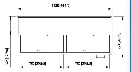
2 **Doors** Capacity 20.1 Cu.Ft. **Dividers** 3 Refrigerant R-290 **Temperature** 33°F ~ 39°F Range Sliding Easy Maintenance **Condensing Unit** 9.8 ft long (3m) flexible three Connection wire cord with modeled plug HP 3/8 Voltage 115V/60Hz **Amps** 3.5 **NEMA Config.** NEMA 5-15 Lighting Interior LED lighting
