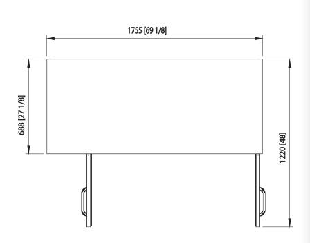
N/A Drawer Capacity 23 Cu.Ft. **Shelves** 4 Refrigerant R-290 **Temperature** 33°F ~ 39°F Range Easy Sliding Maintenance **Condensing Unit** 9.8 ft long (3m) flexible three Connection wire cord with modeled plug HP 3/8 Voltage 115V/60Hz **Amps** 3.8 **NEMA Config.** NEMA 5-15 Lighting Interior LED lighting
