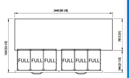
**Drawers** Capacity 21.4 Cu.Ft. Refrigerant R-290 **Temperature** 33°F ~ 39°F Range Easy Sliding Maintenance **Condensing Unit** 9.8 ft long (3m) flexible three Connection wire cord with modeled plug HP 3/8 Voltage 115V/60Hz **Amps** 3.5 **NEMA Config.** NEMA 5-15
