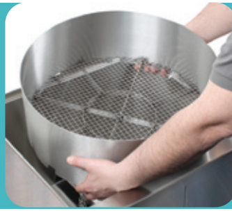
Conveyor easily lifts out for cleaning access.
