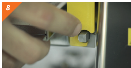
8 Press the lateral button to extract the steel bin. Removable in just one click.
