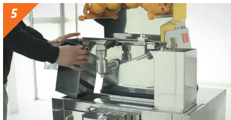
5 Take out the inox peel bucket.
