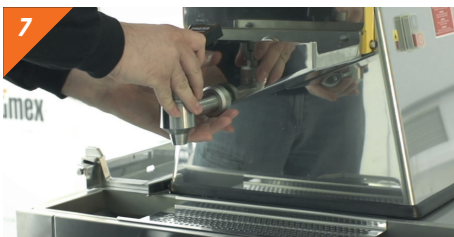
7 Remove the 2Services tap. Easy to dismantle.
